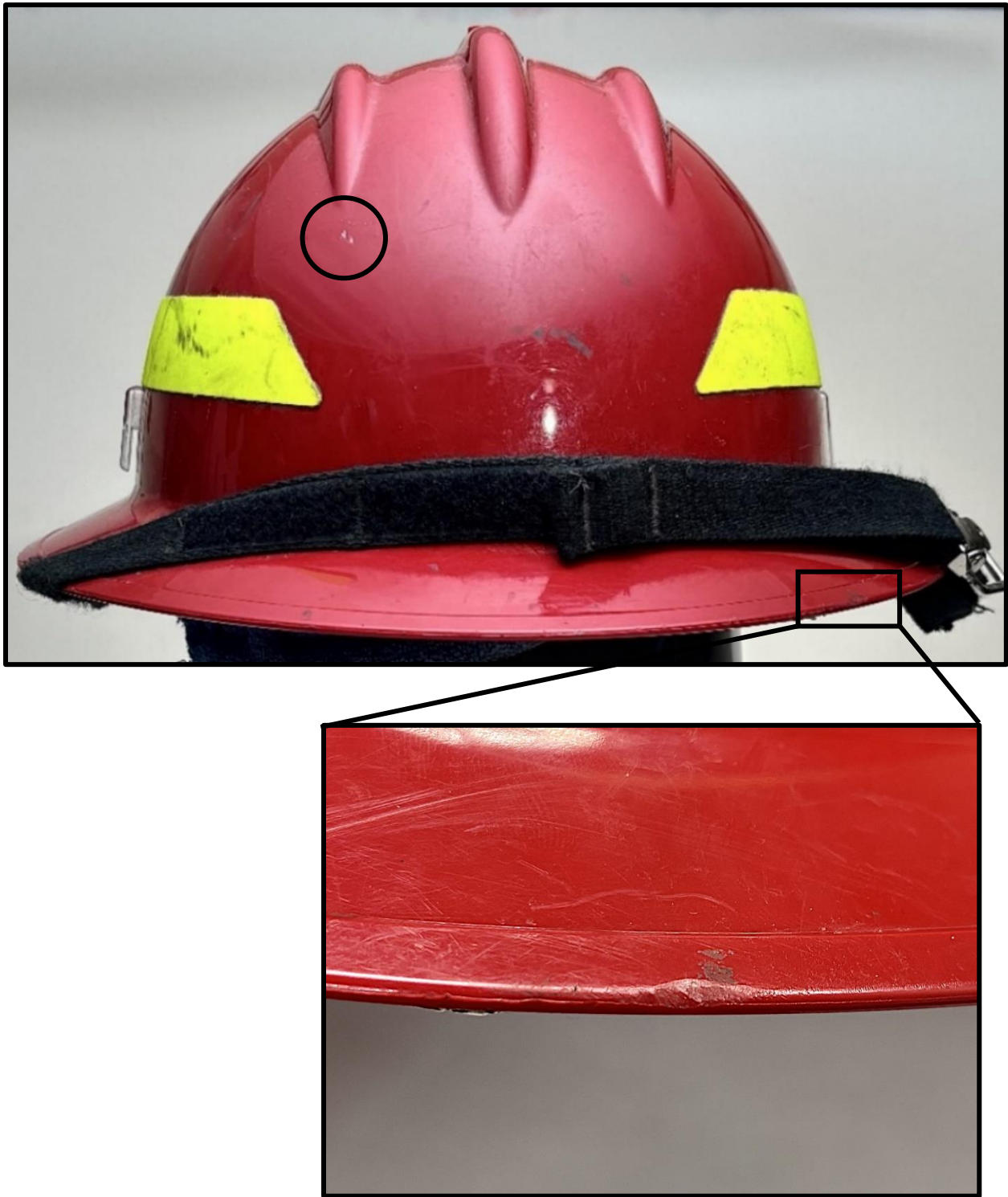
Figure 2: Helmet front showing white scratches (circle), dark scuffing, and brim indentation (box and inset image).
