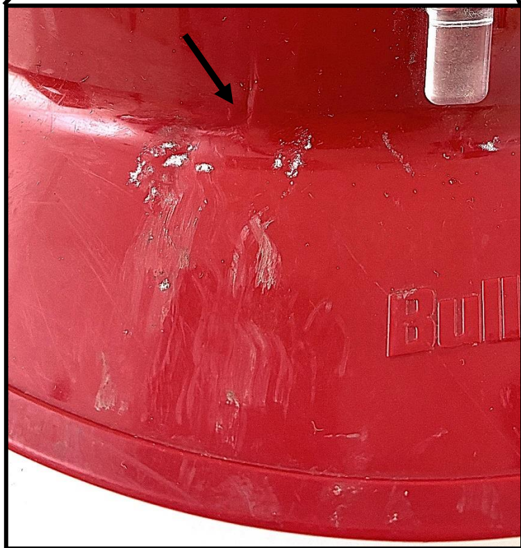
Figure 3: Rear aspect showing dark scuffing, scratching, white gouging, and indentations present. Arrow indicates reverse L-shaped indentation above the brim/cap margin.
