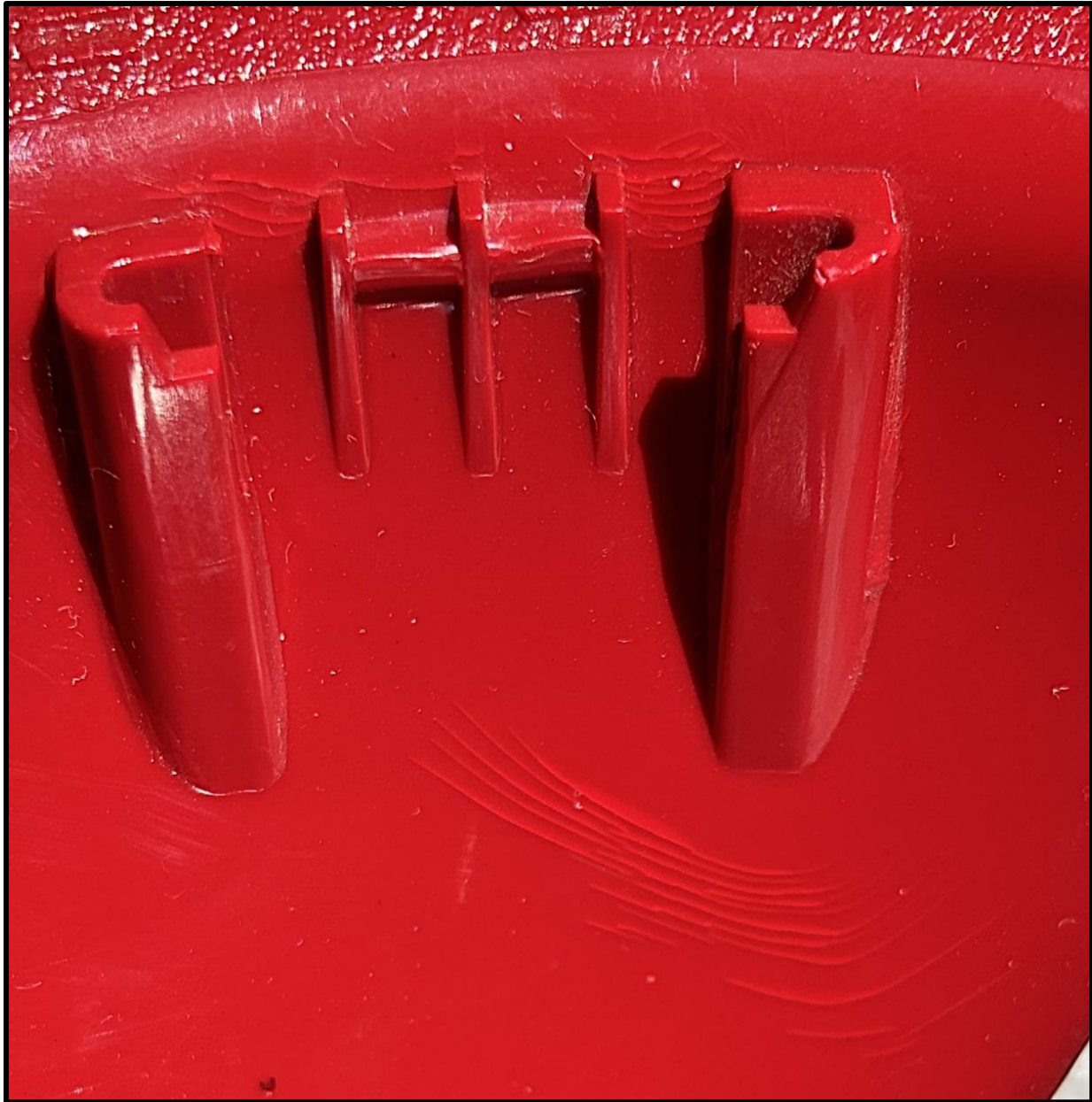
Figure 9: Crazing found above and below the right rear key slot.
