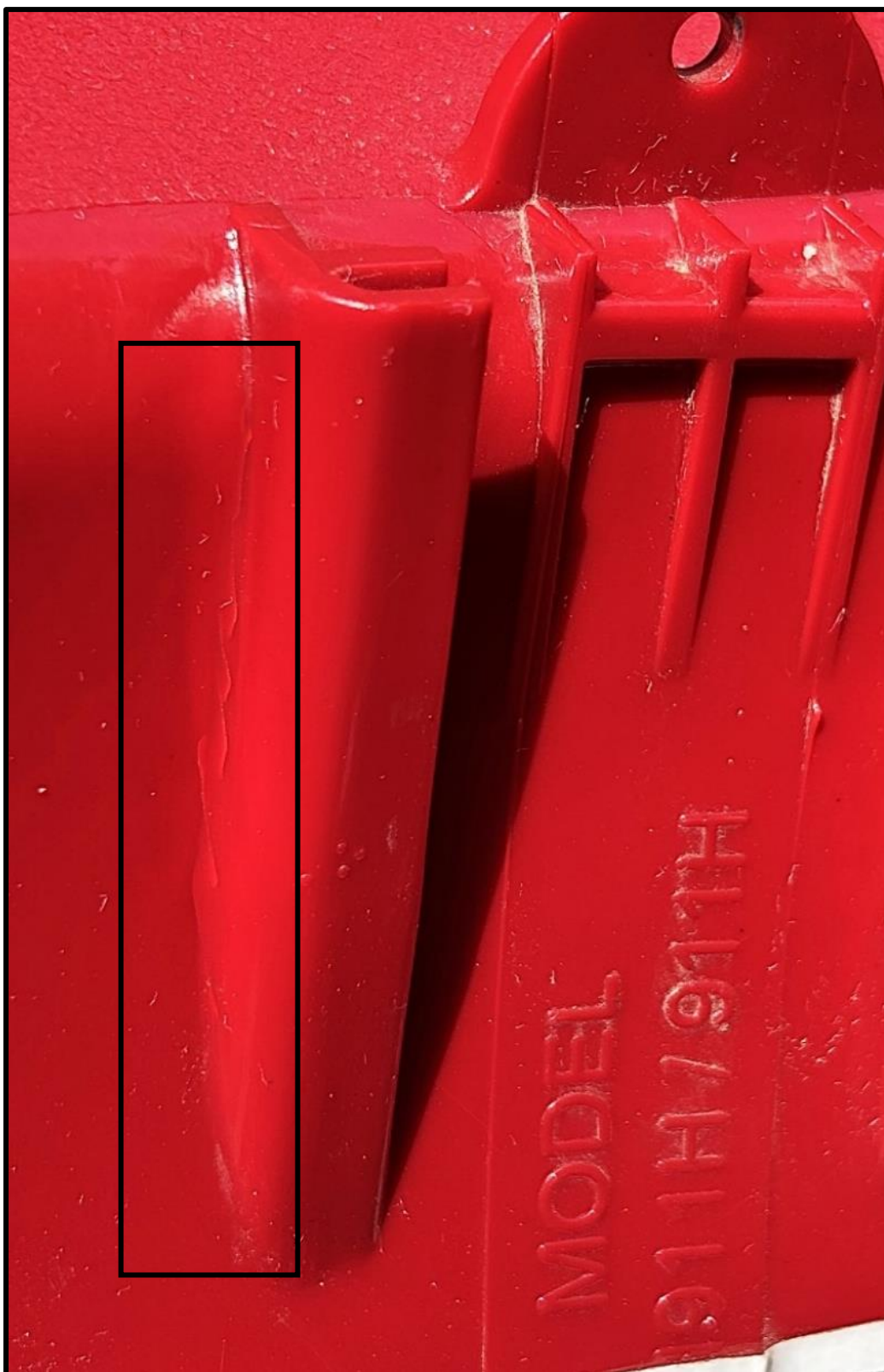
Figure 8: Right lateral key slot crazing where key slot attaches to helmet shell. Shown by rectangle.
