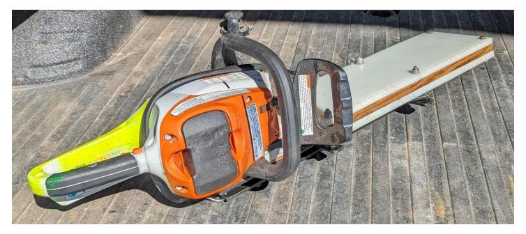
The case material is plastic material with wood there the chain might make contact.
