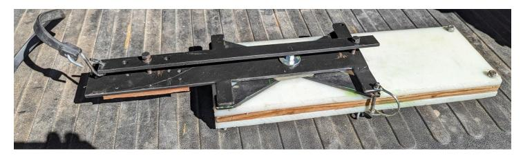
The unit sits on top of the bales of a decker with the mounting bar securing the unit in place. Typically, the carrier is mounted to that the power head rides forward.
