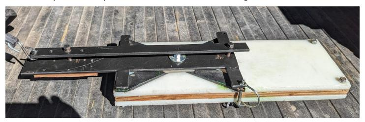
The "X" frame is 7.5 inches  $\times$  10.5 inches and can swivel to make getting the saw in and out easier.
