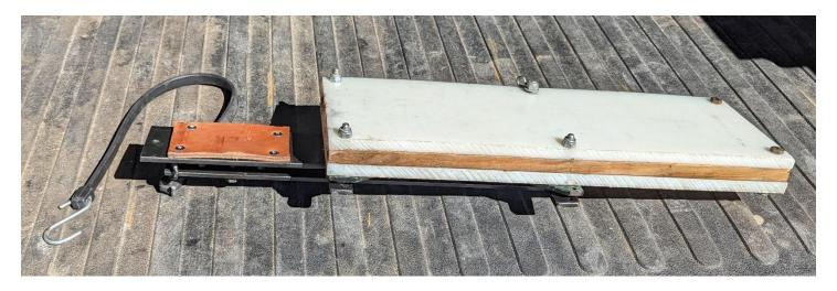
The leather protects the power head from the steel mounting frame.
