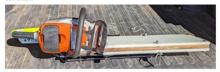
It is designed to carry a 20-inch bar completely protected but will handle up to a 28 inch bar with the tip exposed.
