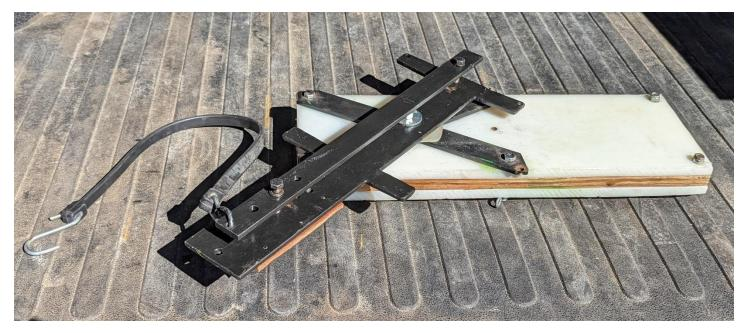
The steel "T" is 18 inches long by 3 inches wide. It is locked in place by a pin when moving down the trail.
