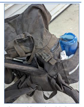
The swamper's line gear that took the direct hit—on the swamper's back—from the 30-foot tall falling snag. Notice how the line gear's hard plastic yoke was blown apart and the hard plastic water bottle was shattered.
