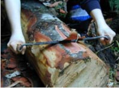
The drawknife is a long, flat blade with two handles on either side. It's used to peel bark off logs. Logs should always be peeled before being used for any construction project. The trick to using a drawknife is to start at just the right angle and draw it toward you while maintaining the angle. If you're good at it you can peel off pieces of bark that run the entire length of the log. If you're bad at it your log will look like it was attacked by a neurotic beaver.
