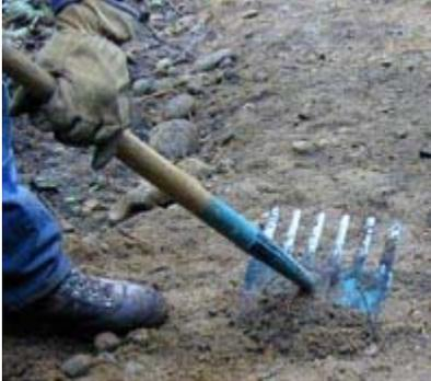
**Usage:** raking, scraping, grubbing, tamping
