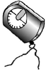
*Tip:* Both eyes must be kept open when sighting through the clinometer.
