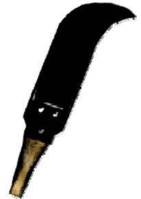
*Safety tip:* Never use an overhead swing. Keep the bank blade in front of you at all times.
