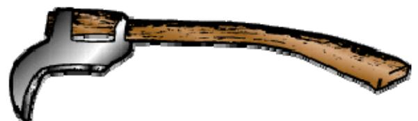
powerful cut. Their curved blades also pose extra safety hazards. Always maintain a firm grip with both hands on the handle. Cut with a slicing rather than a hacking motion and pull back on the handle at the end of the swing to utilize the 12 inch curved blade. Carry brush hooks with the head forward like a shovel.
