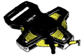
*Tip:* Clean the tape as you rewind it to prevent clogging from debris.
