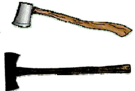
*Safety tip:* Never use a single bit axe as a sledgehammer or as a splitting wedge.
