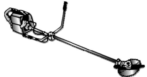
*Safety tip:* The open blade is on the end of a wand, and can snag and swing violently to the side, making it more prone to injure other workers rather than the operator. Other workers should stay clear.
