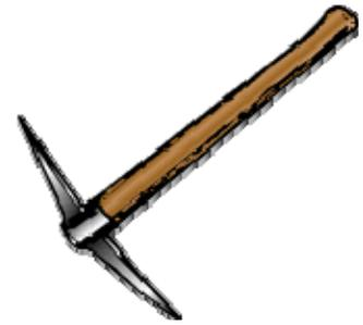
*Safety tip:* Picks should not be used as a lever to pry loose large rock.
