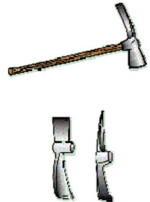
*Safety tip:* The handle can be removed for ease in packing.
