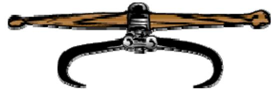
*Safety tip:* A firm tap on the back of the hooks will set the hooks into the log before carrying.
