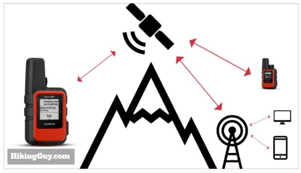
The Garmin inReach Mini works where cell phones don't, using a satellite connection to communicate with other devices, including non-satellite ones like phones and email.
