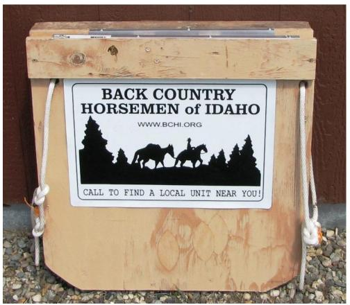
It is very important that the slots you built for the saw blades are big enough for the bar, chain and plastic bar guard. They can be a bit sloppy and the saws will still ride well. I added some metal angle to protect the wood from the saw dogs.
