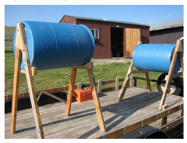
I wanted to keep it simple, but to have a very stable system that would not take much time or cost much to build. I also wanted to keep the cost down. The material to make one of these blue mules includes three 3/8 inch x 48 inch threaded rods, with washers and nuts. Six  $\frac{1}{4}$  x 4 inch carriage bolts with nuts and washers, plus eight screws  $1\frac{1}{2}$  inches long. Four 2x4 x 8 foot long, and some scrap plywood, and one plastic barrel.
