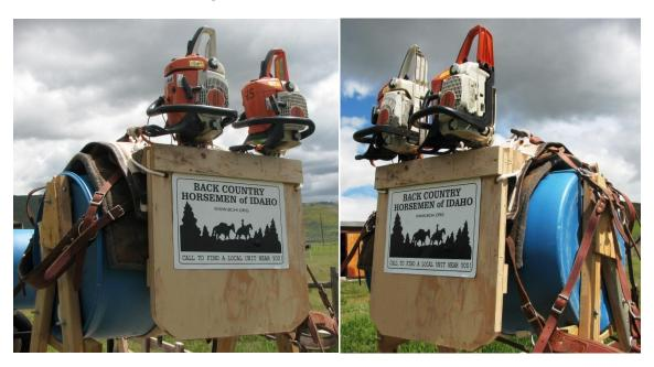
The saws ride very well like this, the engines cool down after use and they are easy to get on and off your stock horse. I don't have any straps on mine to secure the saws, but they could be easily added.
