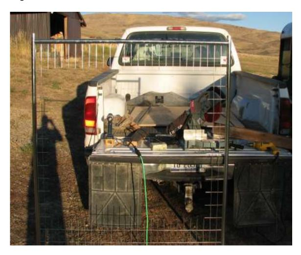
The bottom sits on 2x4 that I secured to the inside of the sides and has a 7/8 hole drilled so that I can remove it easily. I also put 2x4 around the top to add strength and protect the sides from the horses pushing on them. I cut the grill with a saber saw with a metal blade.
