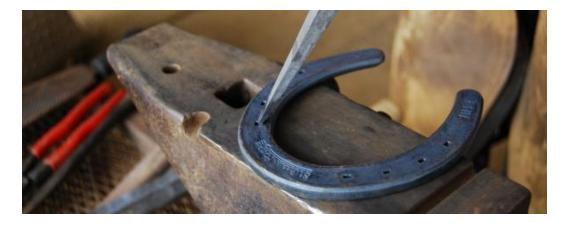
Back-punching is done from the hoof surface of a shoe to enlarge the nail holes. It is another method used to make sure nails seat properly.
