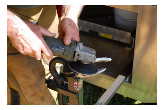
When applying a shoe using an adhesive, Shanks typically uses an aluminum shoe with clips. He first prepares the shoe surface by cleaning it.
